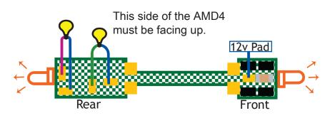
For the extra lighting functions one must use either a 15 mA 1.5v bulb or a LED without a resistor. It is critical that only one bulb or LED is attached to each function, and that any 1.5v bulbs used are rated for 15 mA.
